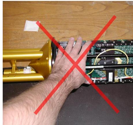
**DO NOT HOLD OR GRAB THE PROBE BY ANY OPTICS, ELECTRONICS BOARDS,
