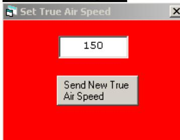
This red box sets your airspeed manually. The airspeed is typed into this box and sent to the probe. The approximate airspeed is necessary to prevent imaging distortions when recording data. The value in this box must be in meters per second. SPEC typically does not manually input the airspeed. On most research aircraft airspeed is available to investigators via a serial string from a COM port or through a second Ethernet card.
